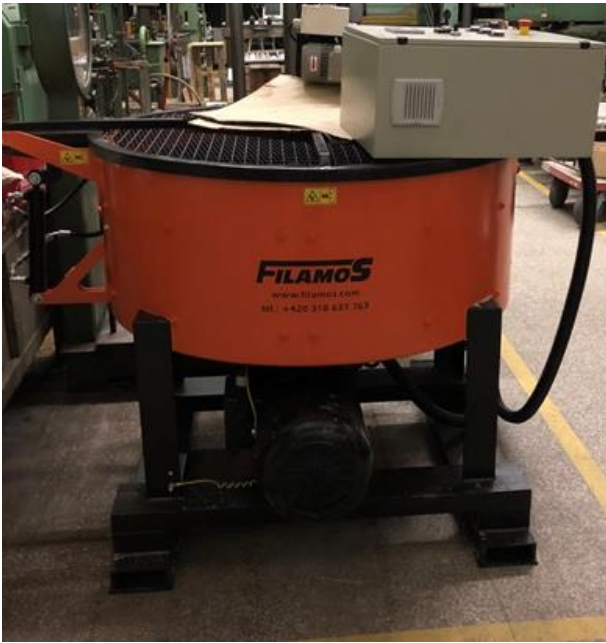
Figure 6. The mixing device with maximum capacity of 200 l
