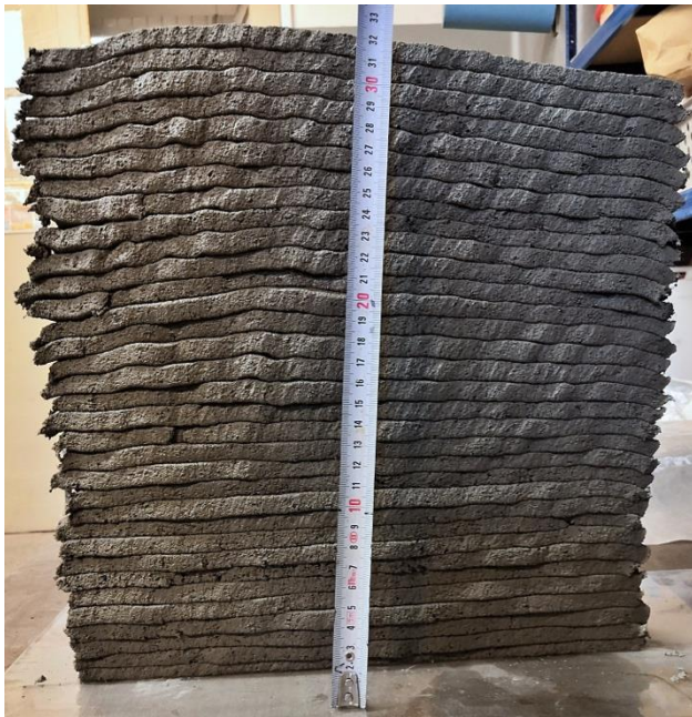
Figure 2. Manually printed cement layers atop each other – pilot tests of buildability
