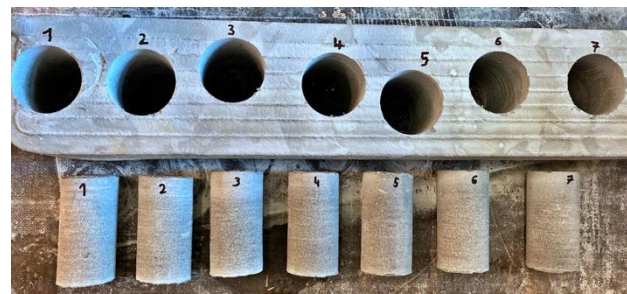
Figure 5. Drilled cores with diameter of 80 mm
