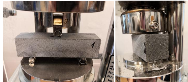
Figure 4. Flexural tensile strength test (left) and compressive strength test (right) on 40x40x160 mm beams
