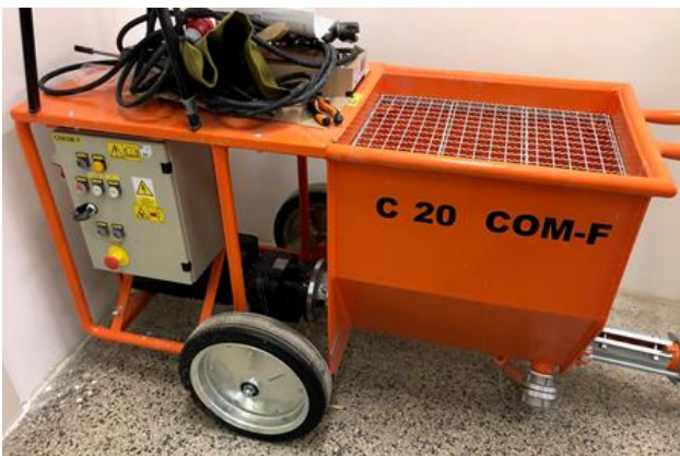
Figure 6. Concrete mixture pump with frequency converter
