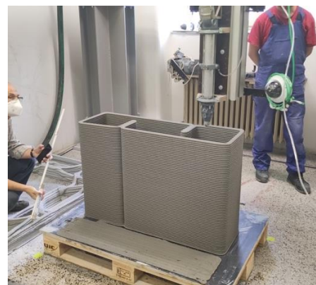
Figure 7. Example of thin-wall object with very short layer times. Extrusion width 20 mm, object height 85cm
