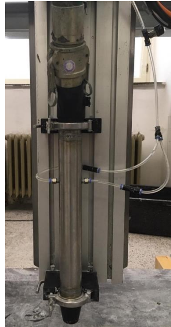
Figure 6. The current printhead with setting accelerator injection, quick-release system
