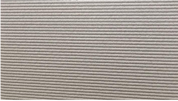
Figure 8. Consistency of surface, layer height 10 mm
