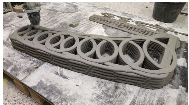
Figure 12. Example of a shape with minimal amount of sharp corners
