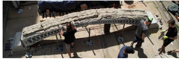
Figure 22. Load bearing test of the experimental footbridge
