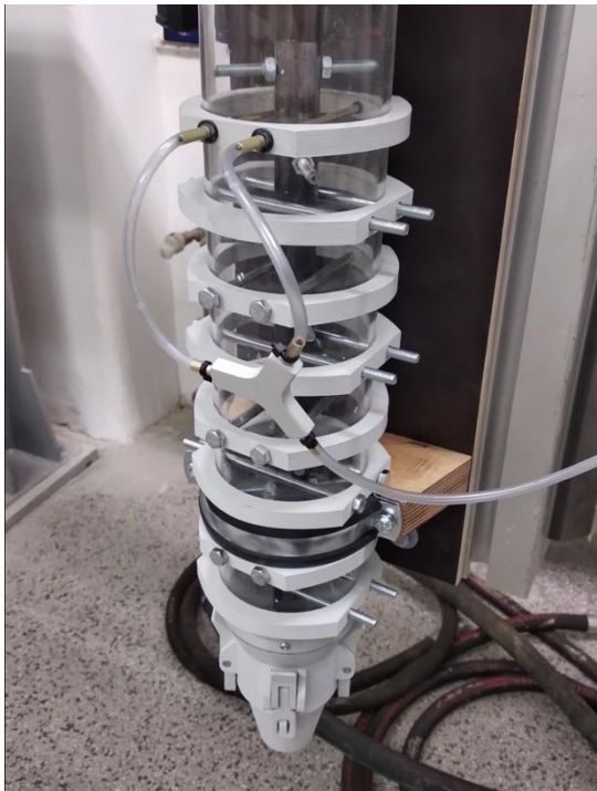
Figure 5. Clear body printhead to visually assess the length of the accelerator mixing path
