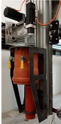
Figure 1. First prototype of the printhead – open system with hopper.
