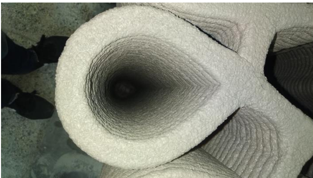
Figure 13. Example of a print where the print path crosses itself in the same layer
