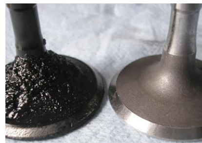
Figure 5. Valves before and after cleaning [BG 2024]
