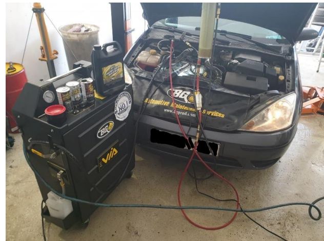
Figure 10. Connection of cleaning machines to the engine
