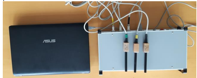
Figure 4. Magnetometer VEMA-040 with probes
