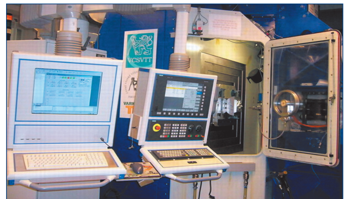
Figure 2. The type LM-2 horizontal three-axis milling machine in the RCMT laboratory.
