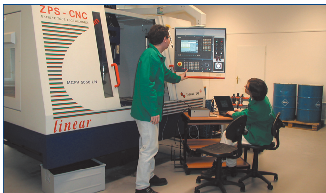
Figure 1. The type LM-1 vertical milling machine in the RCMT laboratory.
