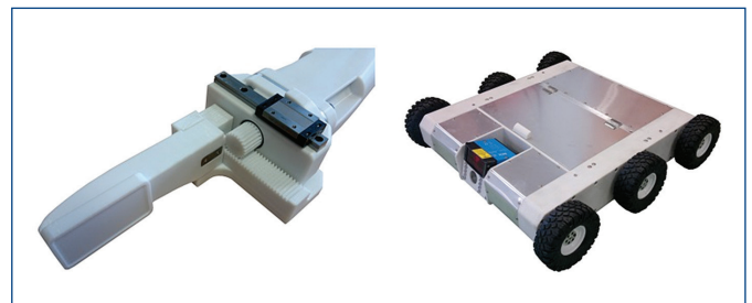
Figure 2: Left –partially dismantled end effector with a visible printed pinion and a rack, right – mobile six-wheel inspection robot Kraken.
