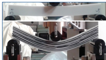
Figure 25. Course of the test in sample type (from top) Solid and Sandwich 8/7
