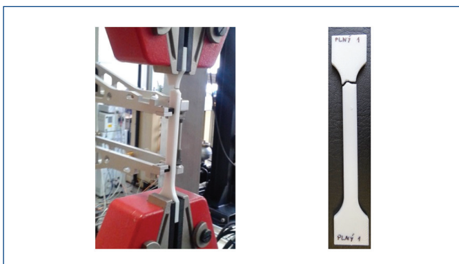
Figure 20. Tensile test of the Solid sample, horizontal
