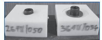
Figure 14. Destruction of sample Sparse M6 – Screw (on the left)/Sparse M6 – Washer L
