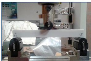
Figure 24. Process of three-point test in flexion, sample (1) (Solid).
