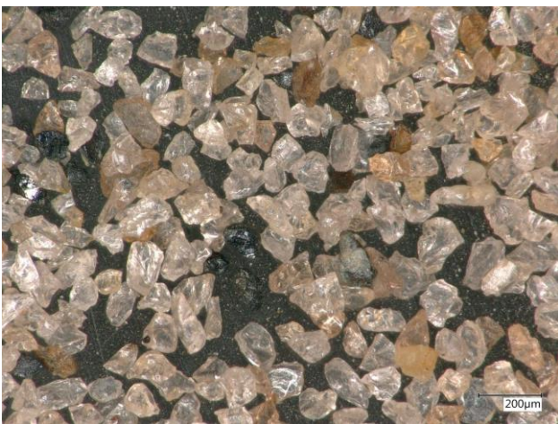
Figure 3. Grains of Australian garnet 200 MESH used during experiments
