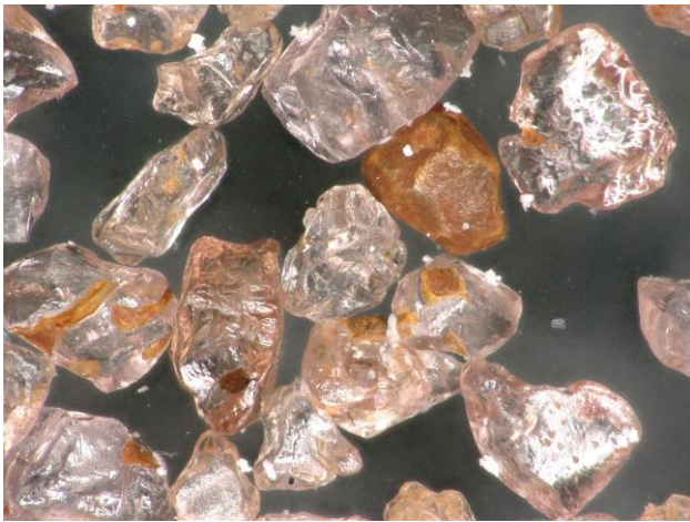
Figure 2. Grains of Indian garnet 80 MESH used during experiments
