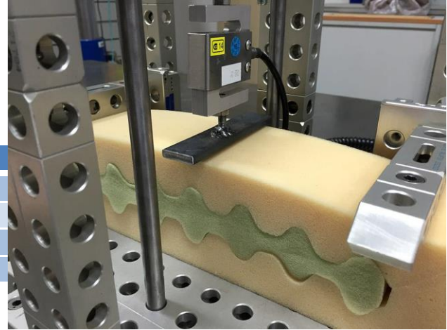
Figure 3. Foam pressing device with a calibrated tensometer
