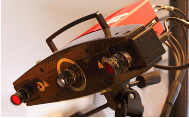
Figure 2. ATOS optical 3D scanner with MV250 measuring volume
