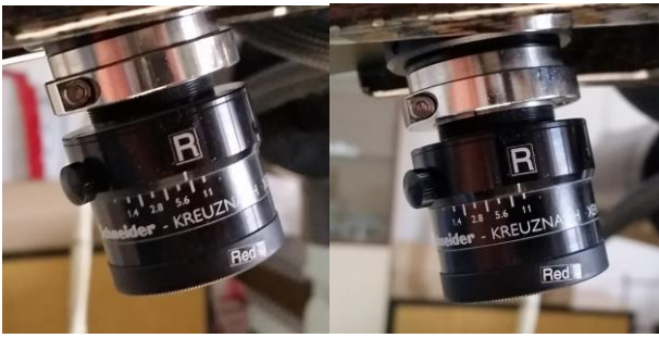
Figure 22. Change of shutter value from 8 to 11 for the right camera (+1 EV)
