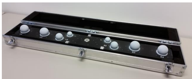
Figure 1. Calibration etalon by GOM for so called Acceptance Test
