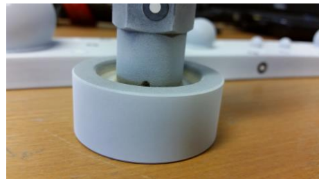
Figure 3. Cylindrical measuring gauge with anti-reflective coating
