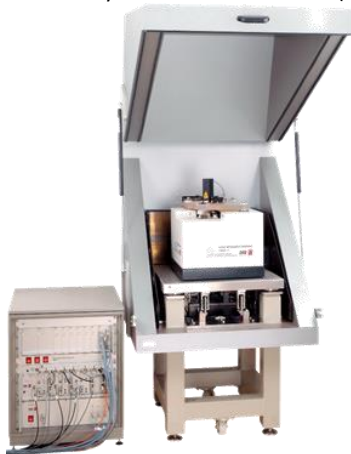
Figure 1. Overall view on the nano-CMM NNM-1 [SIOS 2012]
