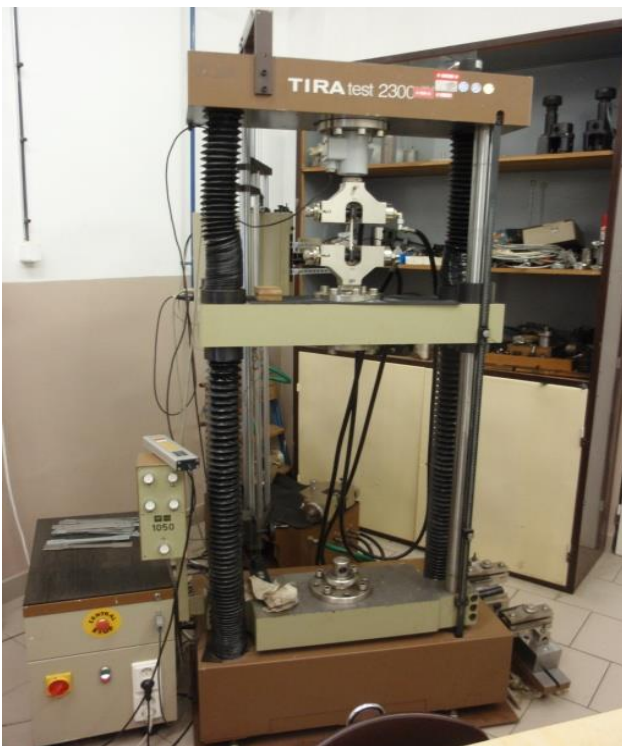
Figure 5. Clamping test sample in the machine
