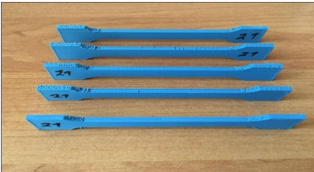
Figure 4. Test specimens made of blue PLA oriented horizontally in length
