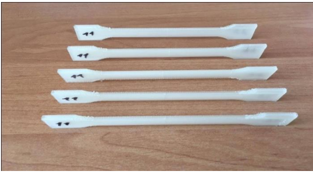
Figure 3. Test samples made of clear PLA oriented horizontally in length
