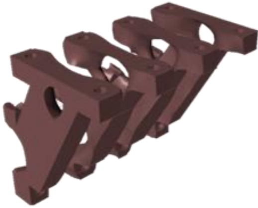
Figure 18. Topology optimization results from Altair Inspire
