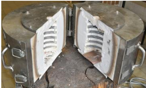
Figure 4. Electric induction furnace M20VA
