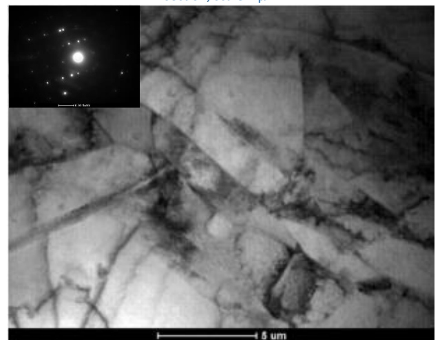
Figure 11. TEM analysis of AZ31 alloy before ECAP - cross section, scale 5 μm
