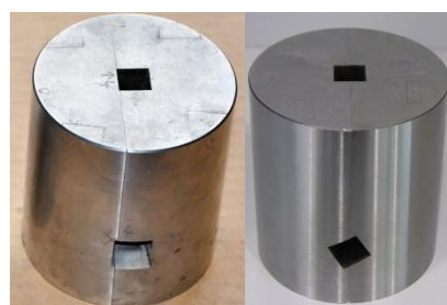
Figure 2. ECAP helix tools: (a) 10°, (b) 30°
