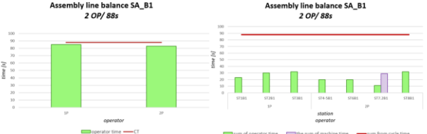
Figure 28. Balance of assembly line SA subassembly B (slow CT – 2 OP) [Klepkova 2022]
