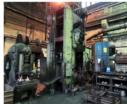
Figure 16. Forging line to forge the contactor forging on the LKM 1600 press
