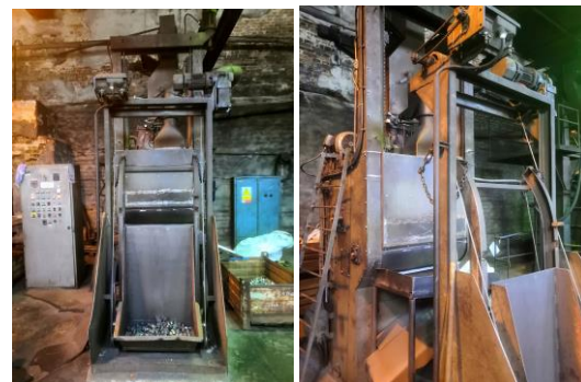
Figure 11. Contactor forging blasting on the BT 63 blast machine
