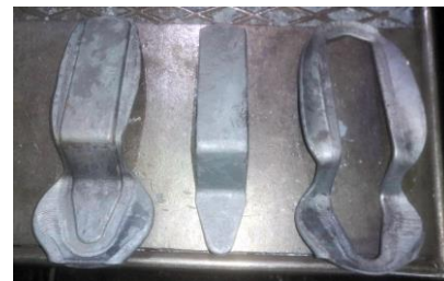
Figure 10. Contactor forging with the material that was in the forging groove (left), sheared forging (centre), and shearing waste (right)
