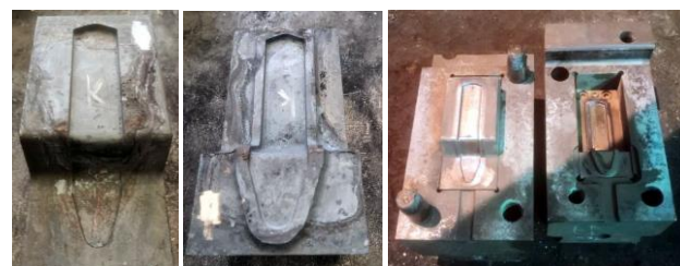
Figure 6. Lower and upper forging inserts and their positioning in the sleeves for forging the contactor forging on the hammer
