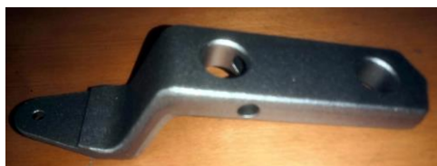
Figure 3. Contactor forging after burr and needle grinding, after blasting, and after subsequent machining
