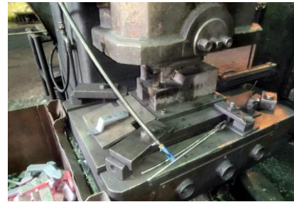
Figure 9. Shearing tool for cutting contactor forgings on the LE 160 shearing press
