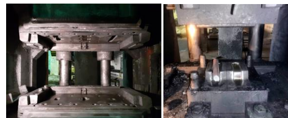
Figure 17. Clamp square sleeves in the LKM 1600 press and insert the semi-finished product into the forging cavity of the die for the production of contactor forging
