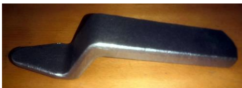
Figure 2. Contactor forging after burr and needle grinding and after subsequent blasting
