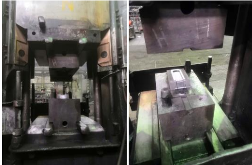
Figure 7. Clamping the lower and upper part of the die to forge the contactor forging on the KHZ 4 A hammer
