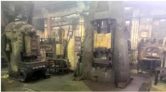
Figure 8. Forging line to forge the contactor forging on the KHZ 4 A hammer
