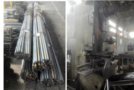
Figure 4. Cutting of metallurgical material into semi-finished products by cold cutting with machine shears ScK 250
