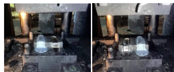
Figure 18. Forging of the contactor forging in the forging cavity of the die fixed in the LKM 1600 press and docking in the die docking cavity
