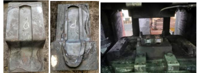
Figure 15. Lower and upper inserts of the forging die to forge the contactor forging on the press and clamping with the wedges of the lower square sleeve with the lower inserts of the die on the LKM 1600 press
