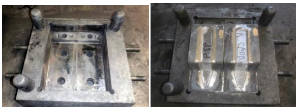
Figure 14. Lower sleeve and lower die with two forging inserts to forge the contactor forging on the LKM 1600 press
