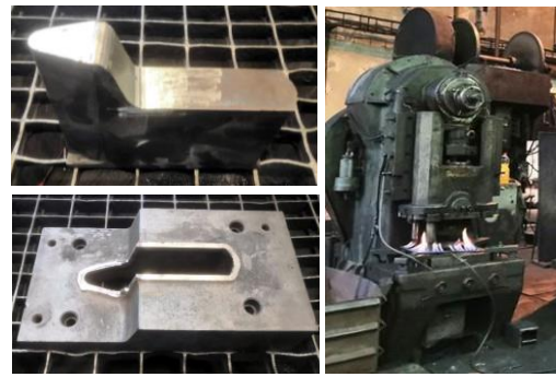
Figure 8. Shear and shear to cut the contactor forging on the LE 160 shearing press
