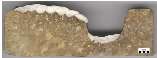
Figure 4. Macrostructure of sample C with the pore
