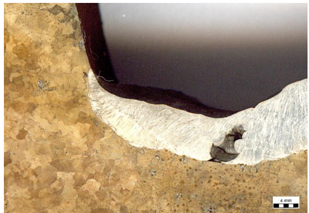
Figure 5. Macrostructure of sample C with the pore and cracks
