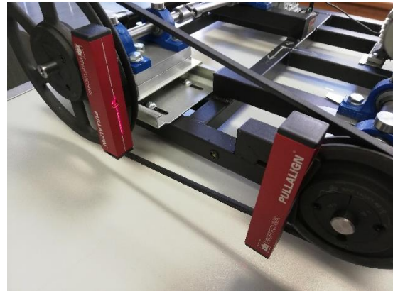
Figure 4. Use of PULLALIGN tool to correct basic angular misalignment
