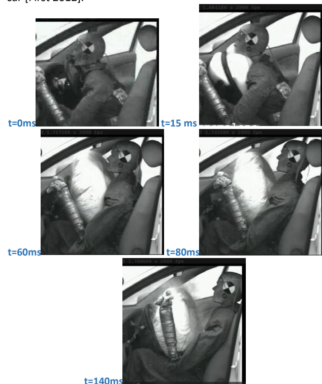
Figure 18. Sequence of the OP airbag test [First 2012].
