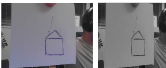
Figure 2. Image preprocessing: on the left is original picture; on the right is picture after applying resizing, auto-orientation, contrast adjustment, and grayscale conversion
