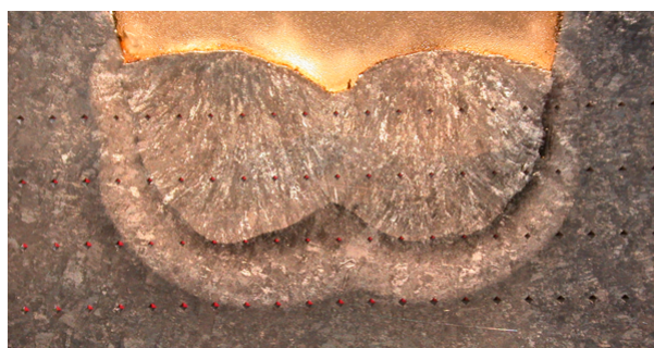
Figure 4. Rows of hardness measuring sticks for first two weld layers
