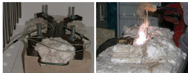
Figure 2. Welding jig with clamped specimen during heating in the furnace (on the left) and isolated during welding (on the right)
