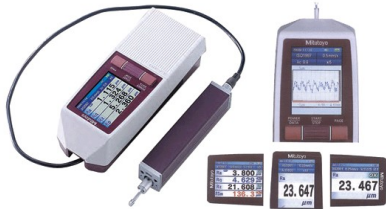
Figure 5. Contact roughness tester Mitutoyo SJ 210 used for experimental measuring the roughness parameter of eroded surface [Gamin 2015]
