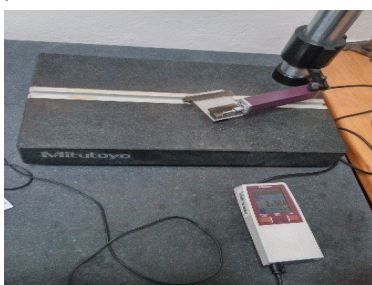
Figure 7. Measurement of roughness parameters of the steel MS1 samples after WEDM
