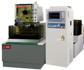
Figure 4. WEDM equipment CHMER G32F used for machining of experimental samples of MS1 material MS1 [Gibas 2009]
