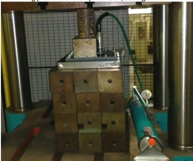
Figure 4. Hydroforming device in hydraulic press [Mrna 2015]
