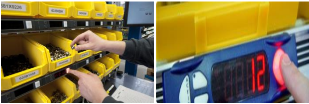
Figure 8. Example of "Pick by light" system [Dematic 2016]
