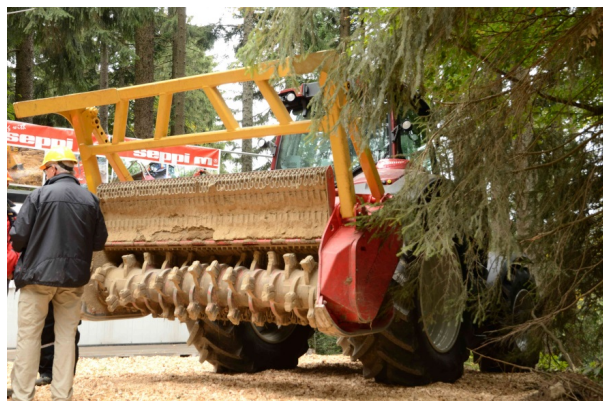
Figure 3. Crusher of undesirable advance growth – additional device
