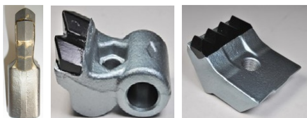
Figure 4. Selected tools a) Single tip [AHWI 2016], b) double tips [SEPMI M. 2016], c) forth tips [AHWI 2016]
