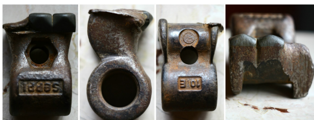
Figure 5. Worn out tool of the crusher of undesirable advance growth
