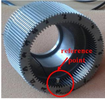
Figure 3. Location of the reference point on the gear wheel
