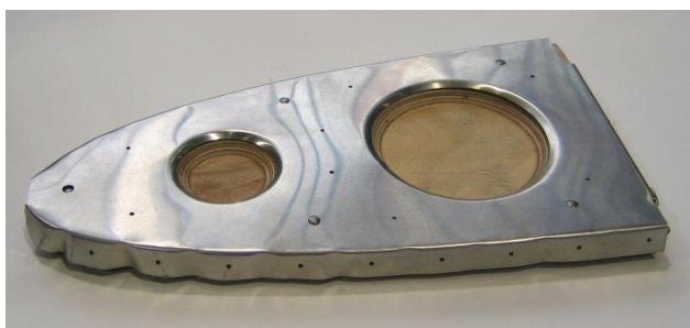
Figure 17. Pressed air rib with punch
