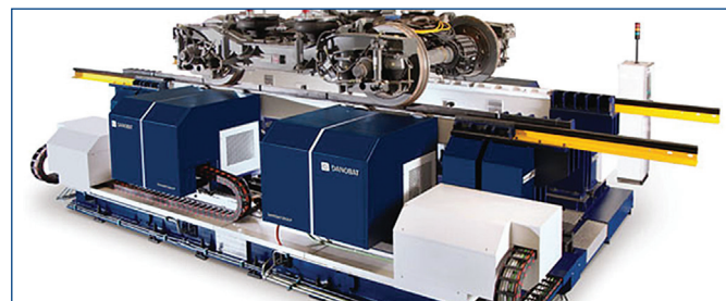
Figure 2. Danobat DTR-25 stand for dynamic testing [Railway Industry Equipment 2014]
