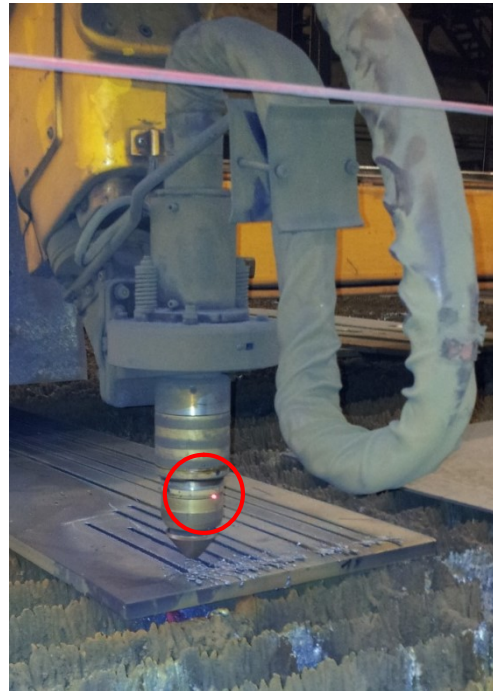
Figure 1. Detail of measuring mechanical vibration at the nozzle head of the plasma machine
