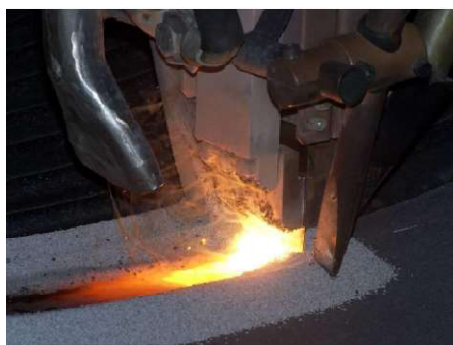
Figure 1. Strip electroslag cladding.
