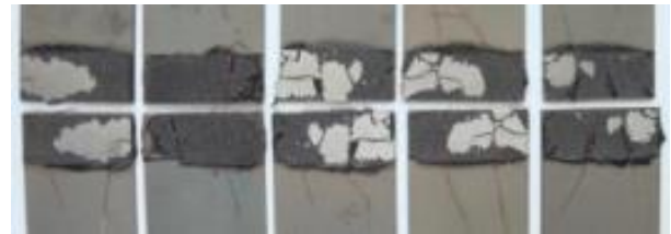
Figure 12. Failure patterns of samples for adhesive A, RT time of heat treatment 16 minutes
