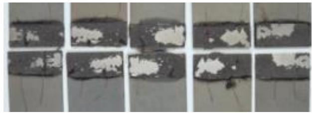
Figure 10. Failure patterns of samples for adhesive A, RT time of heat treatment 12 minutes
