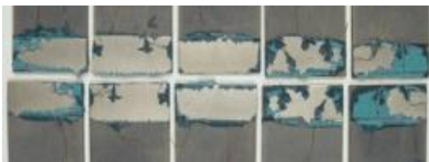
Figure 9. Failure patterns of samples for adhesive B, RT time of heat treatment 8 minutes
