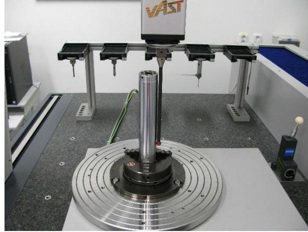
Figure 5. Installed rotary table (RT)
