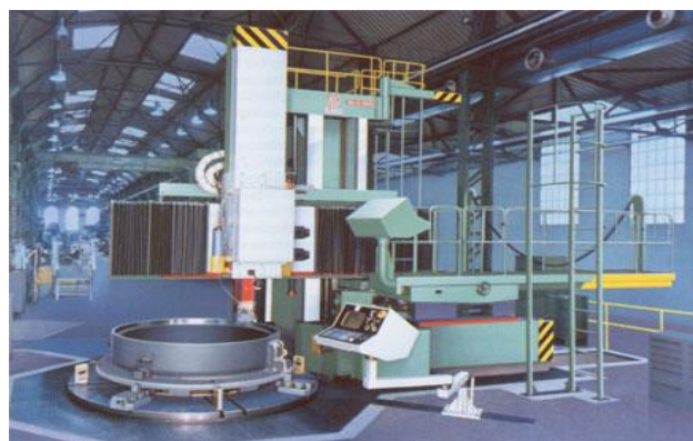
Figure 2. SKJ32-63 CNC, carousel with adjustable rotation axis C [CKD BLANSKO 2017]
