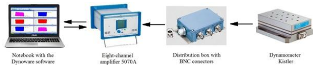
Figure 3. The Kistler data acquisition and processing [Jaros 2015]
