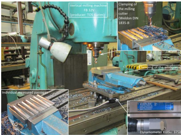
Figure 2. The experimental procedure, clamping of tool and workpiece.
