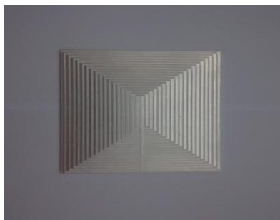
Figure 9. Milling by monolith cutter ø4 mm [Osicka 2017]
