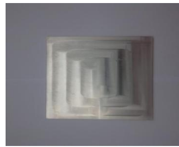
Figure 10. Milling by monolith cutter ø20 mm [Osicka 2017]
