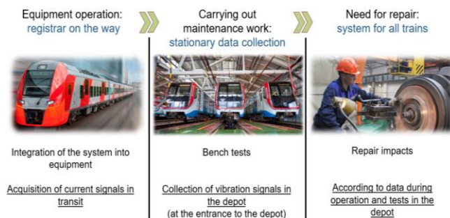
Figure 5. Generalized algorithm for predictive diagnostics of an asynchronous drive of promising trains
