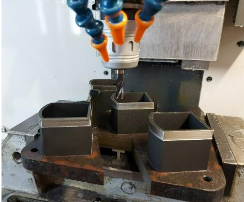
Fig. 3: Outer surfaces finish milling.
