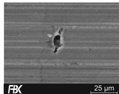
Figure 11: Example of pore on surface of PBF-LB material after milling
