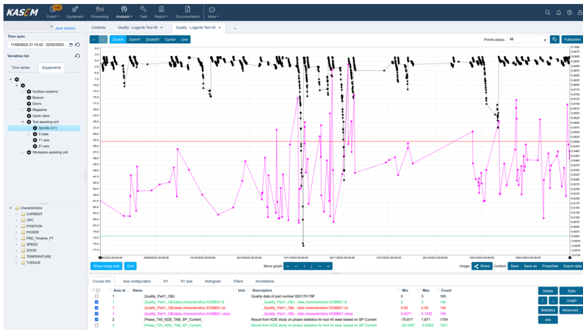
Fig. 14: KASEM® powered visualization of non-quality risk linked with quality measurement - in black the non-quality risk, in pink the quality measurement (in this case the admissible valve seat oscillation 0,05/H1), in red and green quality measurement thresholds.
