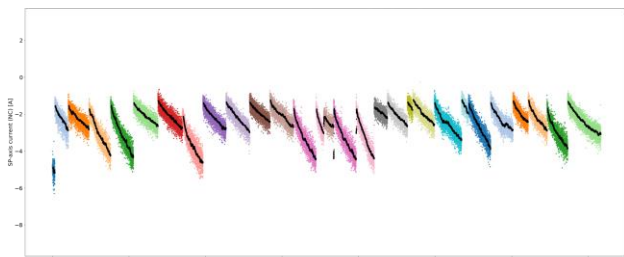
Fig. 9: Tool 45 wear with colored replacements from Spindle point of view.
