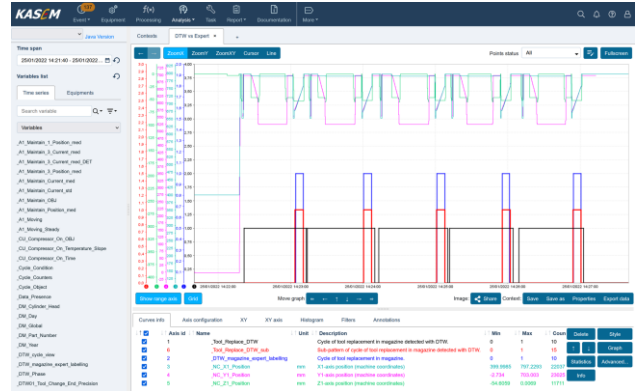
Fig. 7: KASEM® powered visualization of repeated change of tools - in black. The upper part represents the position of the X, Y and Z axes on the machine tool. The lower part represents the sub-pattern presence - in blue the expert label, in red our DTW-based model results.
