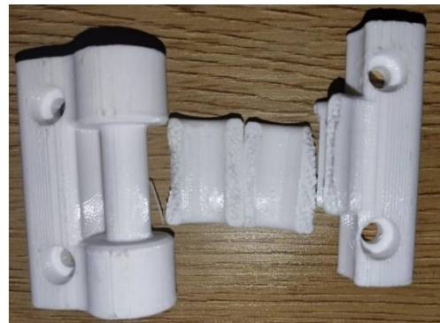
Fig. 14: Hinge with 60% density hexagonal filling.
