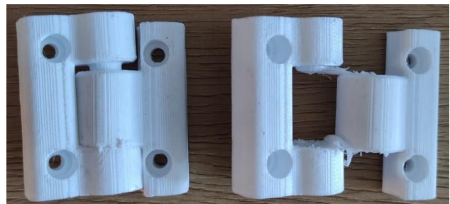
Fig. 19: Hinge damaged by temperature increase.
