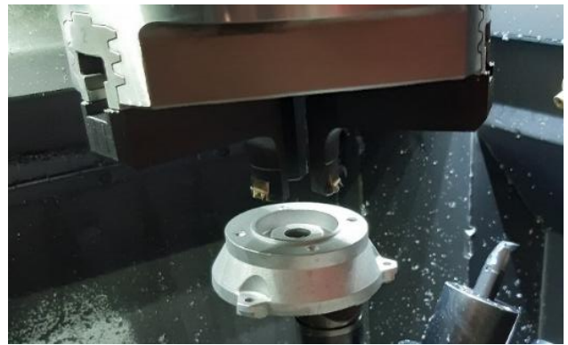
Fig. 16: Clamps before clamping the part.
