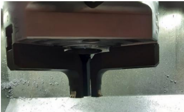
Fig. 15: Chuck with internal clamps.
