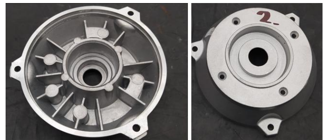
Fig. 5, 6: Machined part of the electric motor - "end-shield".
