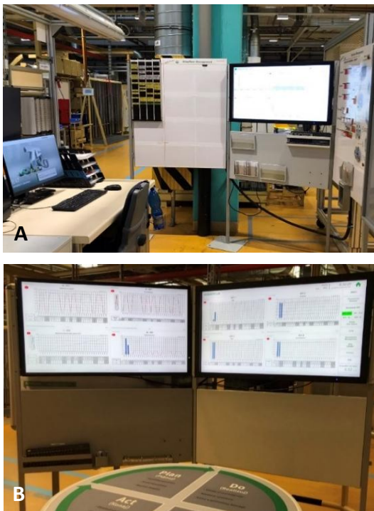
Figure 6. Digitalization of SFM indicators at the level of a) team leader b) production/segment manager [Vizvary 2022]
