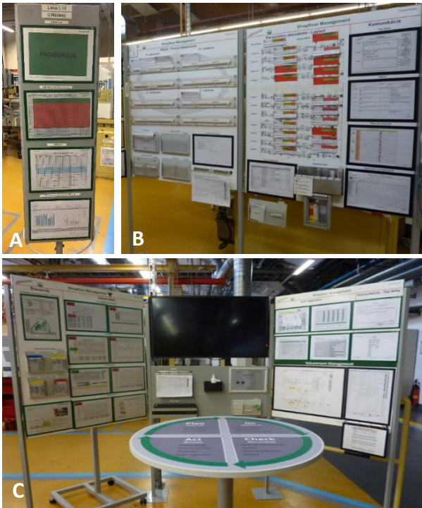
Figure 5. Visualization boards at the level of a) production worker b) team leader c) production/segment manager [Vizvary 2022]
