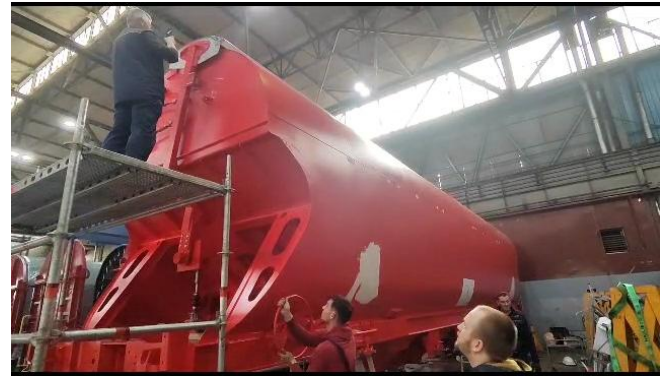
Fig. 10. Input kinematic parameters measurement on the roof mechanism of the wagon
