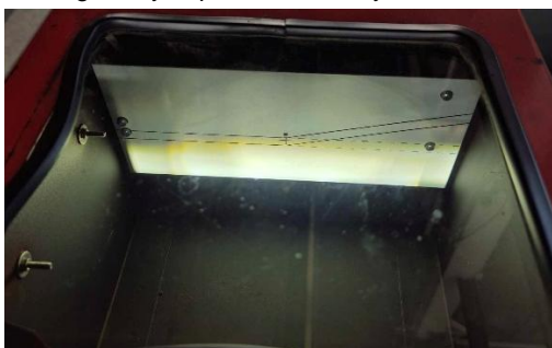
Fig. 10 Reticle of the regloscope using LED headlight (Low beam)
