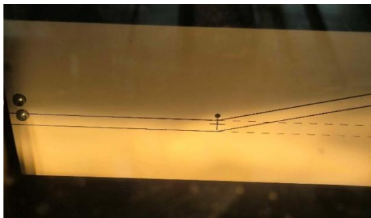
Fig. 9 Reticle of the regloscope using LED headlight (Low beam)
