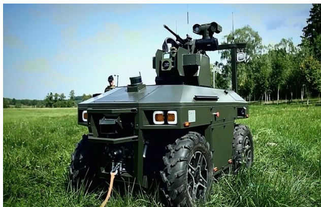
Figure 2. Example of autonomous platform developed on ATV basis: PERU(a), PAWO(b)
