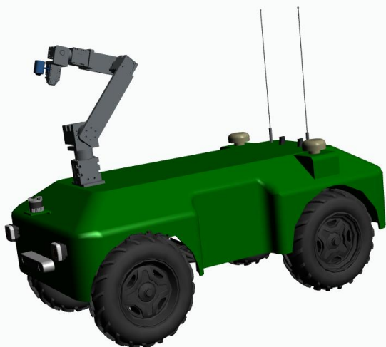
Figure 6. View of integrated modular arm with Unmanned platform
