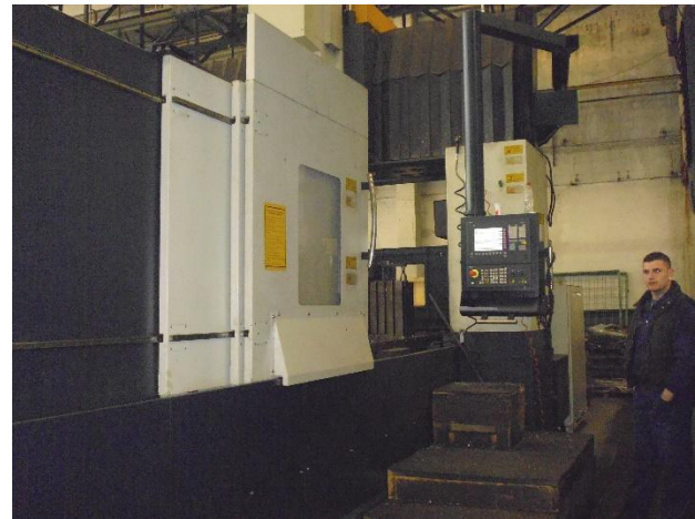
Fig. 7: Selected machine Four star Taiwan FD3242 [28]
