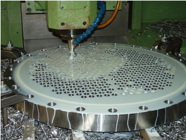
Fig. 8: Application of coolants and lubricants in the process of tube sheet production [29]
