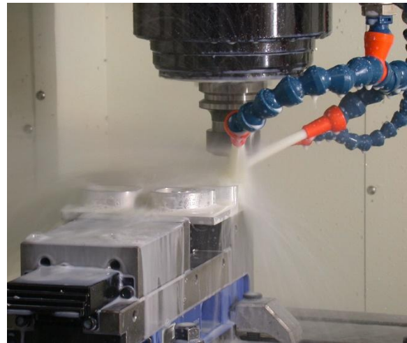
Fig. 4: Example of applying cooling and lubrication during drilling [25]
