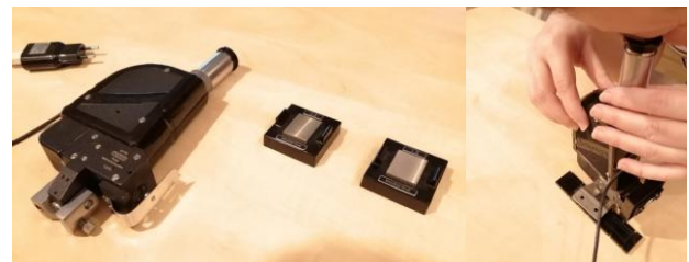
Figure 8. Optical comparison method using a microscope.
