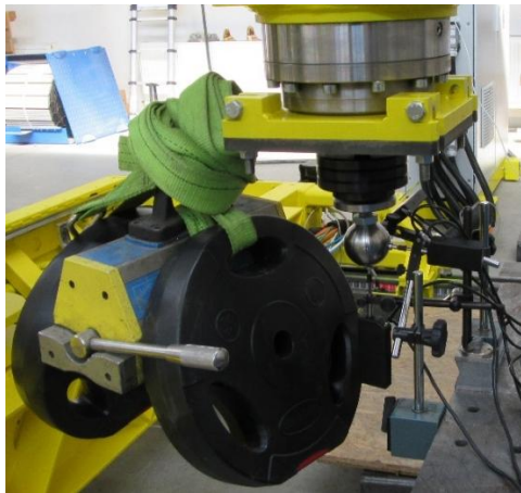
Figure 4. Load placement 100 kg (50% load capacity of the robot)
