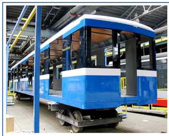
Figure 18: Final configuration of the hybrid body of underground railway car on transfer bogies
