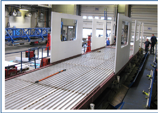
Figure 16: Static strength demonstration tests of the body
