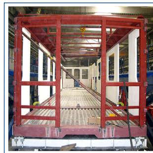
Figure 10: Welded steel nose
