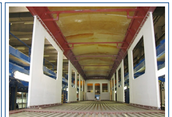
Figure 15: Interior of the completed body shell
