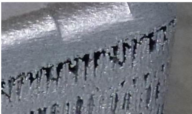
Figure 2. Model 1 – problem with the support structures
