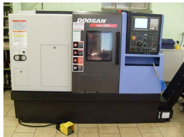
Figure 8. CNC turning machine DOOSAN Lynx 220L
