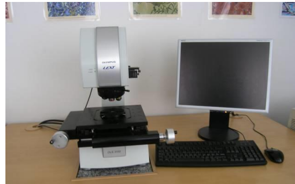
Figure 1. The laser confocal microscope LEXT OLS 3100
